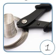
1-Choose the appropriate color and size of Memory wire for your creation. Use the cutters to cut the desired length, but add a few more centimeters in view of the manipulation required when finishing your project.
