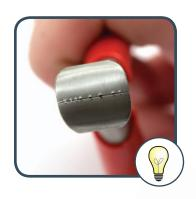
Be careful with your cutters! Sometimes the components of the Memory wire are stronger than those of your cutters. As a result, some cutters will keep permanent marks after use. That's why we recommend working with cutters specially made for Memory wire.
